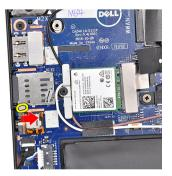
2 Slide the dummy SIM card tray out of the system.
